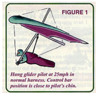
Hang glider pilot at 25mph in normal harness. Control bar position is close to pilot's chin.
