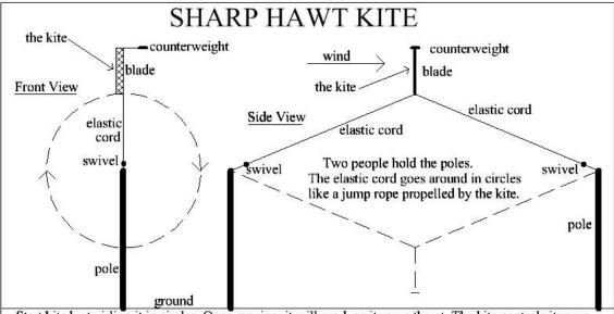
Start kite by twirling it in circles. Once moving, it will produce its own thrust. The kite controls its own pitch angle. The principle of pitch control is called the "T-Rule".
