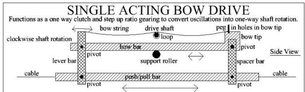
1,000 rpm is easy to achieve with a small shaft diameter. My proof-of-concept model can reach 3,000 rpm, but the braided nylon fishing line bow string begins to heat and fray at that rpm.
