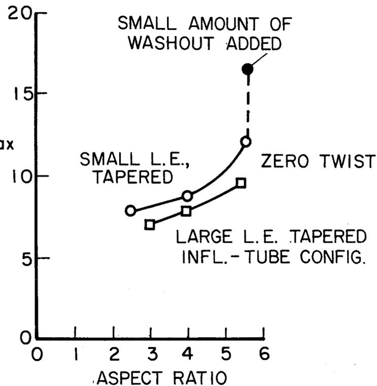
Figure 3.- Effect of aspect ratio on maximum lift-drag ratios of  $50^\circ$  swept flexible wings having rigid frames.
