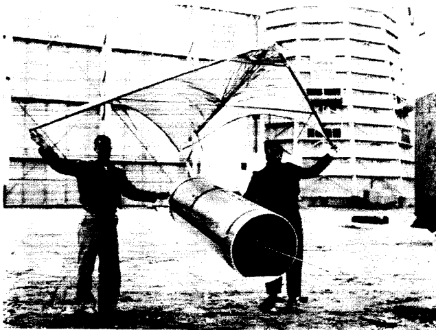
Figure 5. - Paraglider booster-recovery model that was radio-controlled after drop from a helicopter by the Langley Recovery Systems Branch.
