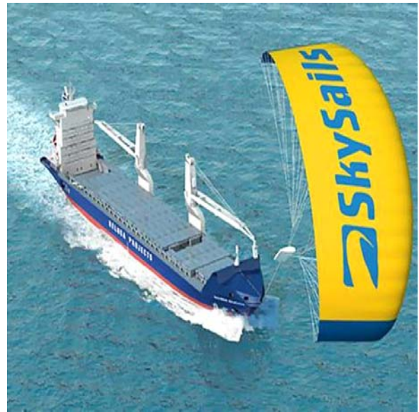
Figure 2. The Skysails system in which a parafoil pulls a ship. ( http://www.skysails.info ).
