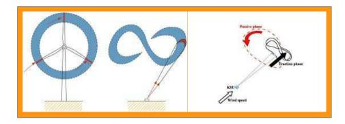
It will look like "Ground jan - Monotethred" (ground generator with one single cable) that the "active phase" of an alternating cycle, said "YO-YO", will generate electricity from the wing traction, carrying the cable from a coaxial drum to a motor-generator positioned on the ground.
