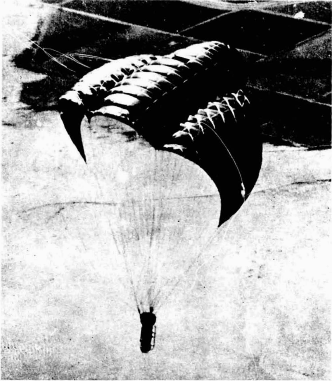
Figure 100. Test 206T parawing in gliding flight, showing some of the canopy damage.
